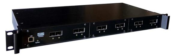
Warning, do not exceed the SFP manufacturer's maximum receive power specification. APD receivers commonly used in long range and tunable transceivers are easily damaged at power levels above -7dBm.
